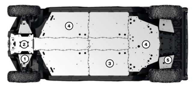
For ultimate durability and strength, all our Aluminum Skid Plates are made with High Strength 5052 H32 Aluminum 3/16" (4.5 mm) thick.
